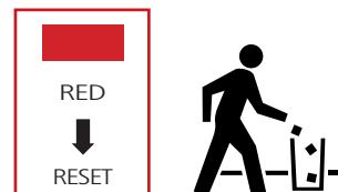
If the colour of the viewing window changes to red, the SPD was overloaded and must be replaced.
